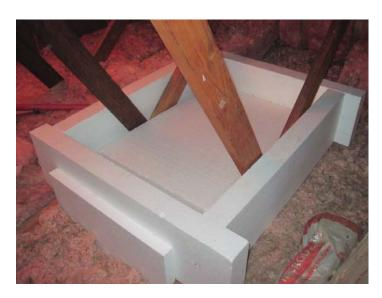
The Energy Guardian® Universal Hatch Cover insulates attic access panels of various sizes while also providing easy access to the attic for the homeowner. The unit is installed in the attic and requires no modifications to the living space area. When assembled, the kit has maximum outside dimensions up to: 10" H x 32" W x 36" L (inside dimension are up to 10" H x 28" W x 32" L).
