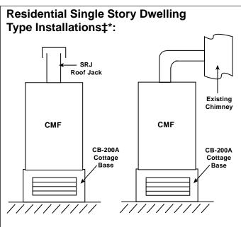
NOTE: Direct Vent Kit may be installed on either the right or left side of the furnace. \* For Non-Manufactured Housing Applications Only.
