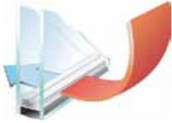
Energy transfer thru full metal spacer
